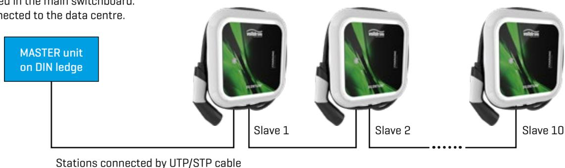
For large installations with a greater number of charging stations, the system can be expanded with group switchboards, which also include, apart from the power supply for charging, a group control unit. The control unit is connected to the MASTER unit by a data cable [Ethernet] and controls the group of charging stations via the RS485 industrial bus. Each group switchboard enables connection of up to 12 charging stations.
